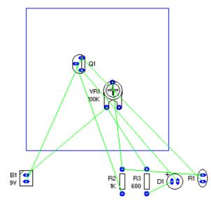
The first step in the conversion process is for an outline of the board to be created. This is shown on the left as a blue rectangle.
