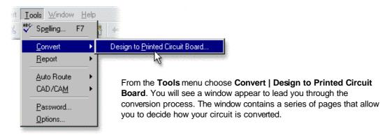
These pages cover areas such as the size and shape of your PCB layout, which components are used as well as more advanced features such as automatic routing and component placement.
