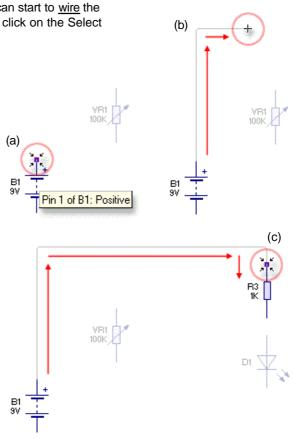
Now a second wire from the top of variable resistor VR1 to join with the wire you have just added.
